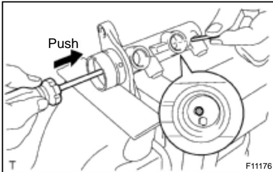
(b) Using a screwdriver, while pushing the No. 2 piston and spring, then install the straight pin.
